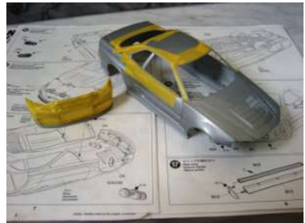
Masking window trims and front bumper spoiler
