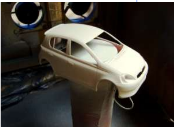
Undercoated in Plastikote white primer
